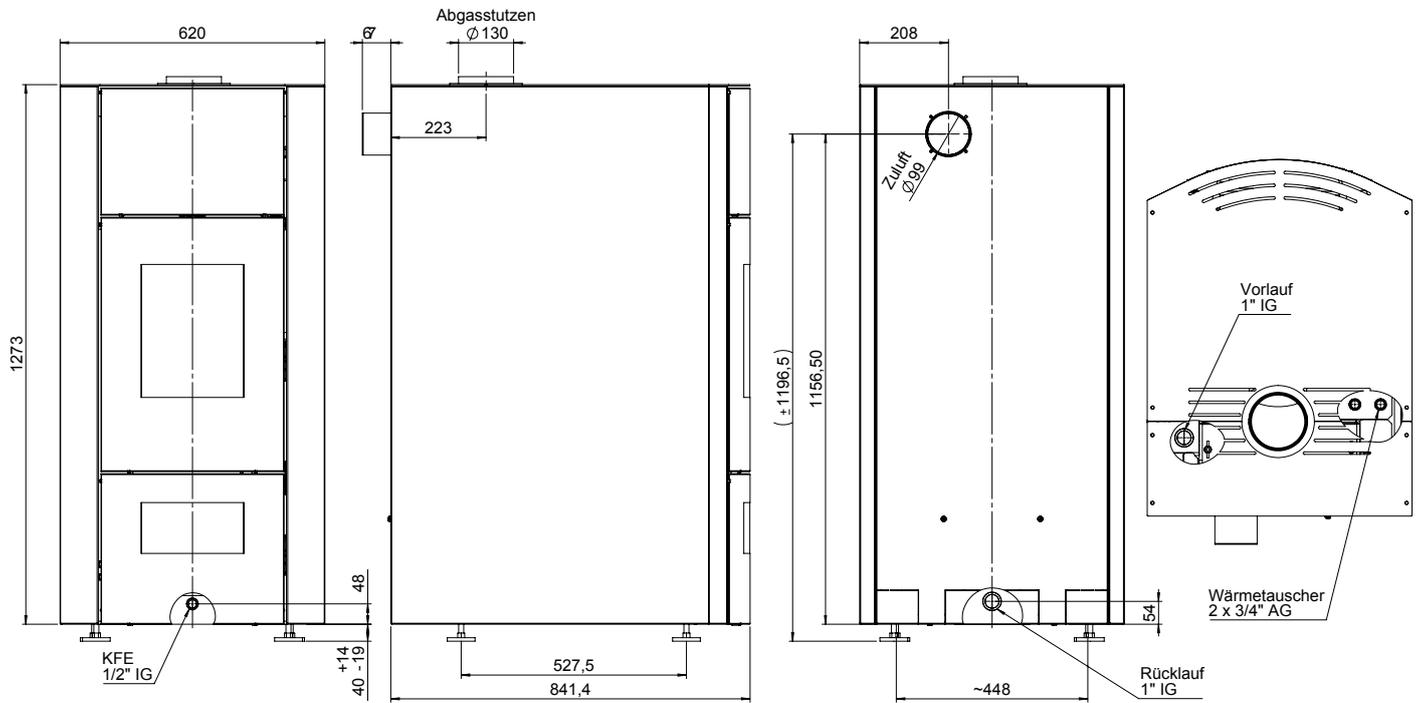
Abb. 40: Abmessungen HV-W / HV-H
